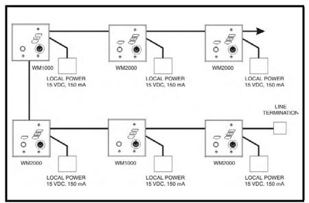
**FIGURE 5.** Locally powered intercom system
